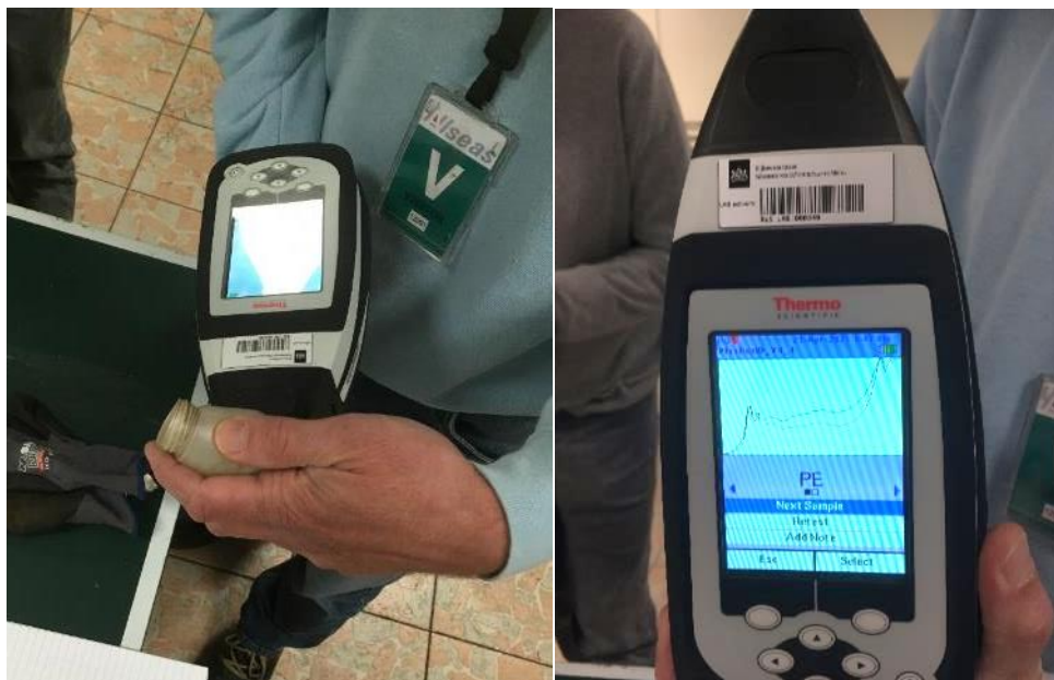
Figuur 6-10: Handheld NIR-spectrometer. ThermoScientific microPHAZIR.
